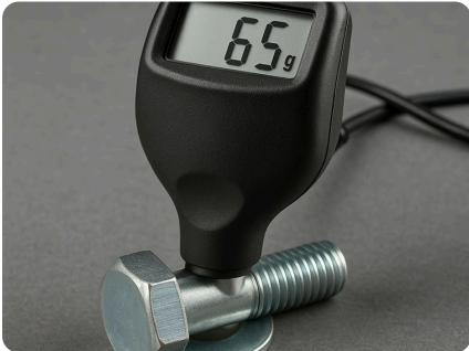
Coating thickness check
